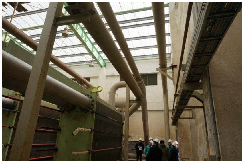
Figure 1: Plate heat exchangers in Asia Symbol Pulp and Paper factory in Rizhao
