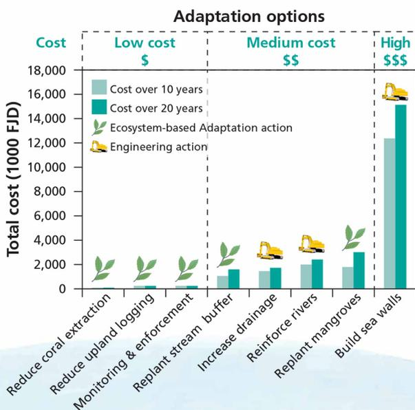
The least-cost alternatives for storm protection include reducing coral extraction, reducing upland logging, and monitoring and enforcement, while the most expensive option is to build sea walls. The medium cost options include replanting stream buffers, increasing drainage, reinforcing rivers, and replanting mangroves. In addition to life-cycle costs of adaptation options, benefit-cost calculations should integrate estimated benefits of avoided damages or ecosystem services.
