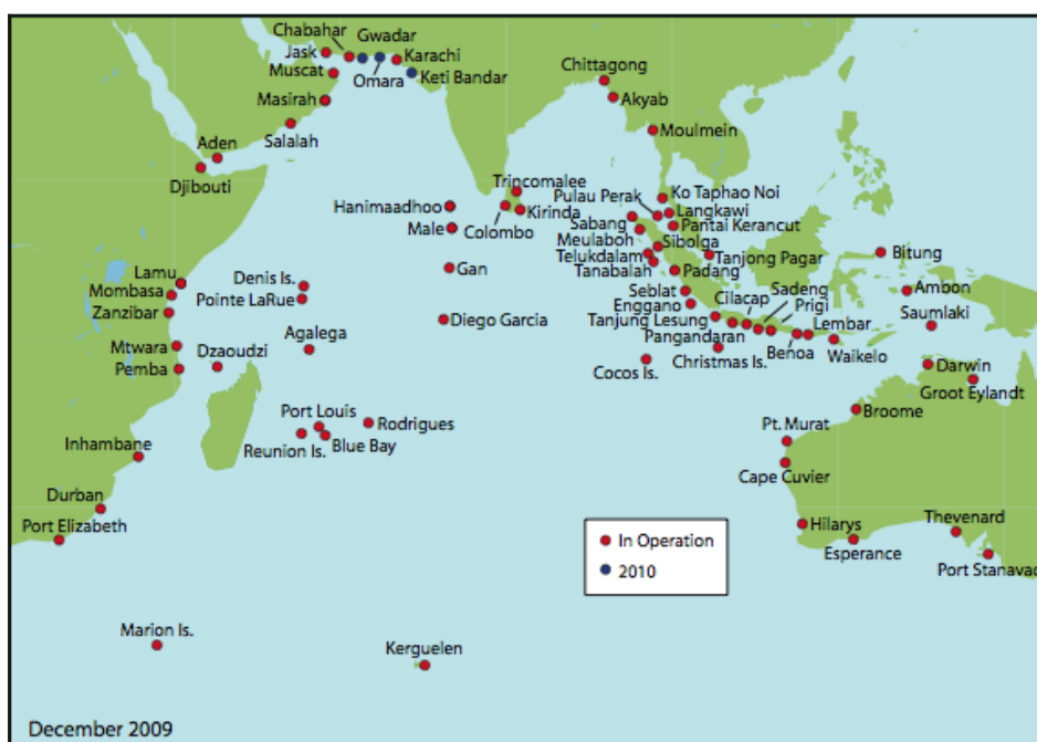
Figure 9: Core Sea Level Network of the Indian Ocean Tsunami Warning and Mitigation System (IOTWS) 42
